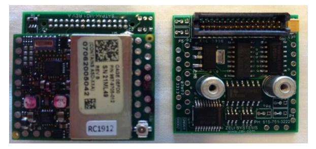
MicroGRAM Attached to Component Side of SATPAK-MG
